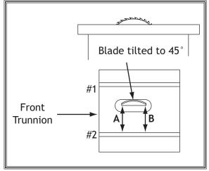
**Figure 98.** Locations of the front trunnion shims.
